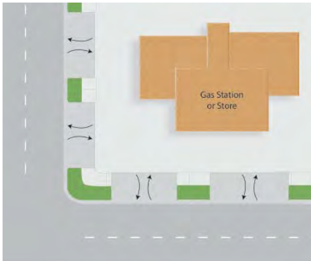
Corner with many wide driveways (Credit: Michele Weisbart)
